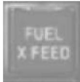
On the right hand side of the engine instruments the fuel X-Feed advisory light is located. In case X-Feed is activated this advisory light illuminates.
